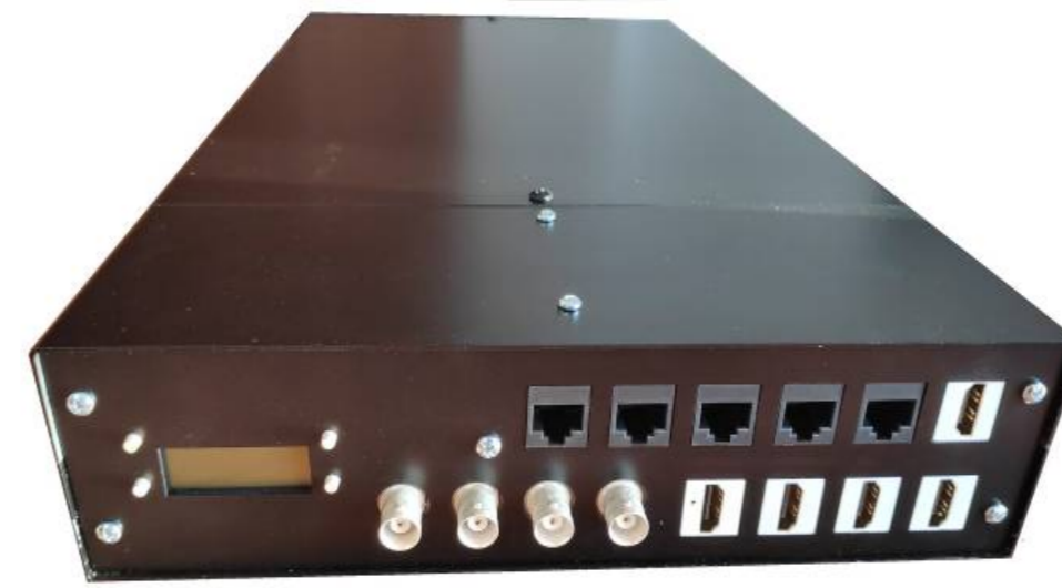
Fig.1. The housing complies with the standard AMC cassette with a communication module with increased mechanical resistance
